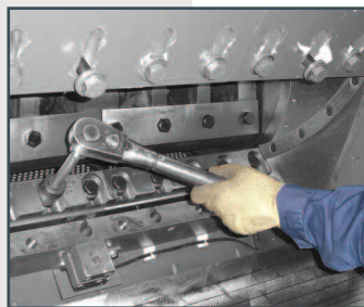
Ease of access and maintenance with front hopper access door
