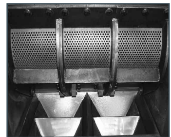
Standard tangential cutting chamber can be modified for bed knife placement to suit changing and demanding production requirements
