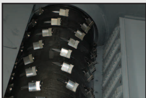
Standard hardened rotor with replaceable cutters and cutter holders designed for high throughput of the toughest materials
