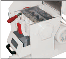
Heavy-duty HCHC/D2 steel construction rotor and knives for consistent, high quality regrind
